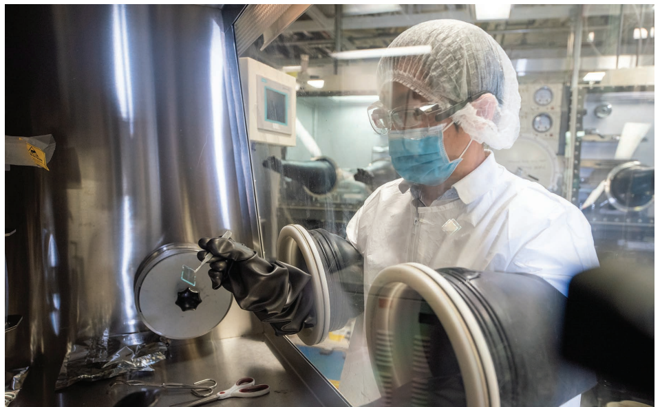
Bin Liu, a postdoctoral researcher in electrical and computer engineering, loads the mirror-like photonic structure into the glove box—on the way to adding the light detector on top of the structure. Photo: Silvia Cardarelli
