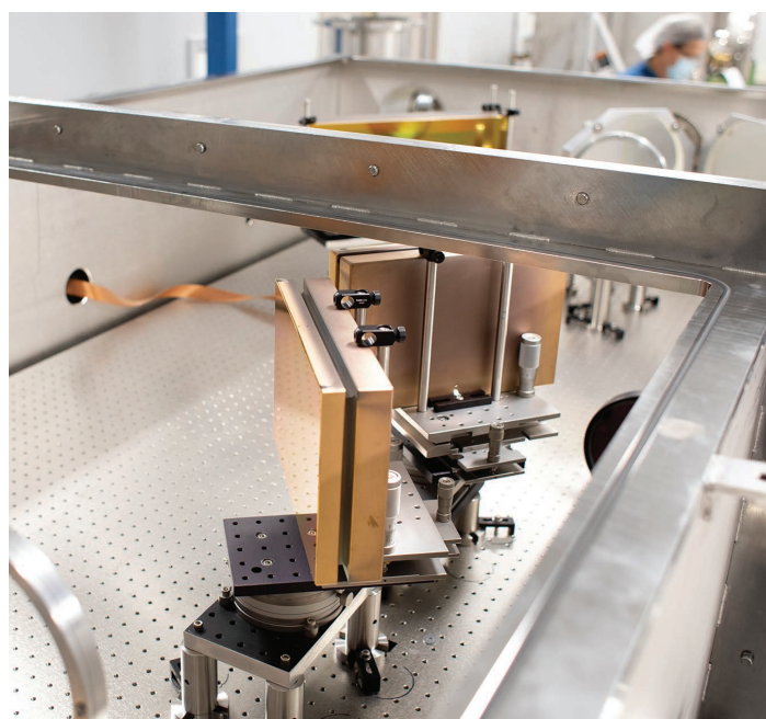
Above: A look into the 500 TW compressor vacuum chamber. Coming soon is the 3PW system.
