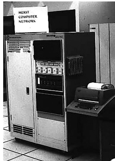
Fig. 2: Merit Network PDP-11 based Primary Communications Processor (PCP) with custom high speed communication and IBM I/O channel interfaces. This photograph was taken on the 2nd floor of the University of Michigan Computing Center Building, Ann Arbor, MI, circa 1975. Credit: Merit Network, Inc.
