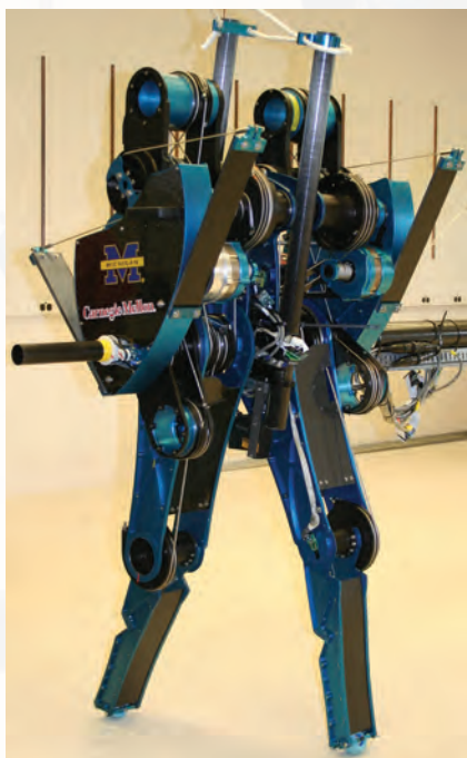
MABEL, a novel robot that incorporates unilateral springs for shock absorption and energy storage. The robot is one meter tall at the hip and weighs 56 kg.
