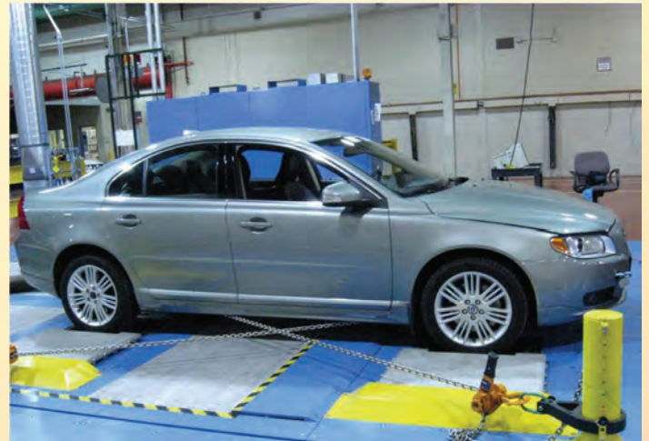
Hybrid electric vehicle testbed for enhancing fuel economy and drive quality.
