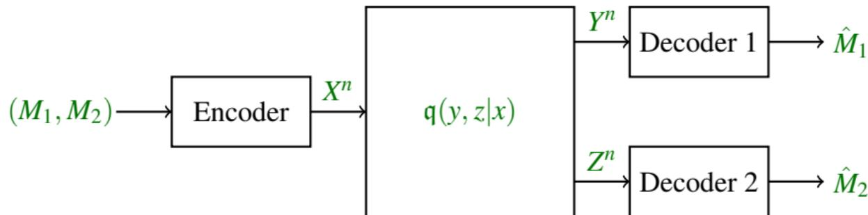
Figure: Discrete memoryless broadcast channel
