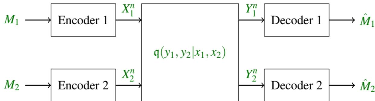
Figure: Discrete memoryless interference channel
