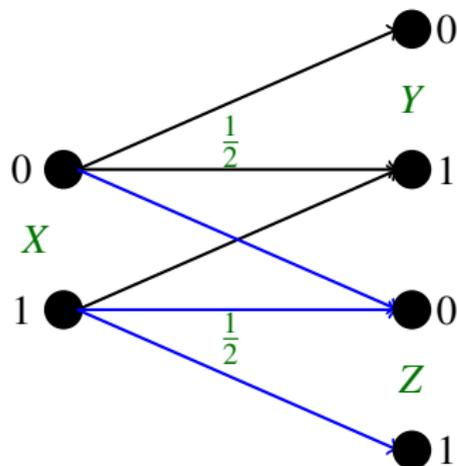
Figure: Binary skew-symmetric broadcast channel
